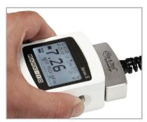
The Plug & Test<sup>®</sup> connector locks into the re-ceptacle in the indicator when fully inserted. Dual buttons on the indicator housing release the connector for easy removal. Gold plated spring contacts ensure long lasting and reliable connection.
